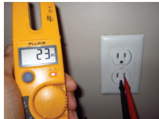
Fig. 1: Identification of ungrounded 3-prong receptacle with receptacle tester
