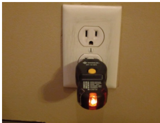
Fig. 1: Identification of ungrounded 3-prong receptacle with receptacle tester
